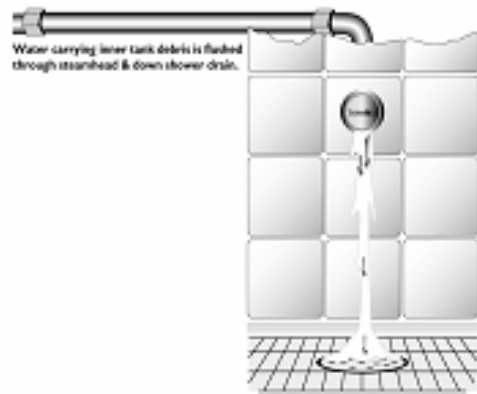
Figure 4: Tank maintenance - power cleaning the tank.
