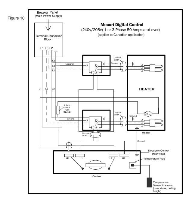
CAUTION: THE MANUAL RESET LIMIT SHALL BE WIRED IN THE CIRCUIT.
