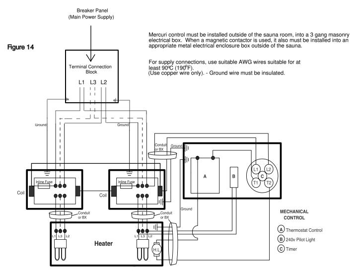
CAUTION: THE MANUAL RESET LIMIT SHALL BE WIRED IN THE CIRCUIT.
