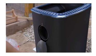
Insert the Chimney adapter into rear hole tapping with a rubber mallet until it is snug.
