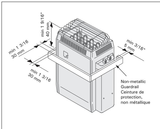
Figure 8. Safety railing of the heater
