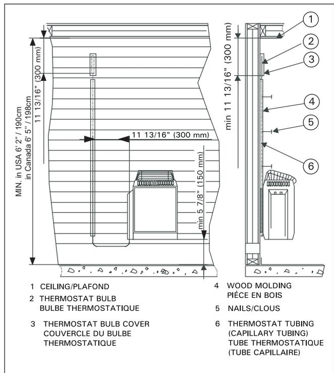
Figure 7. Installation of the thermostat sensor
