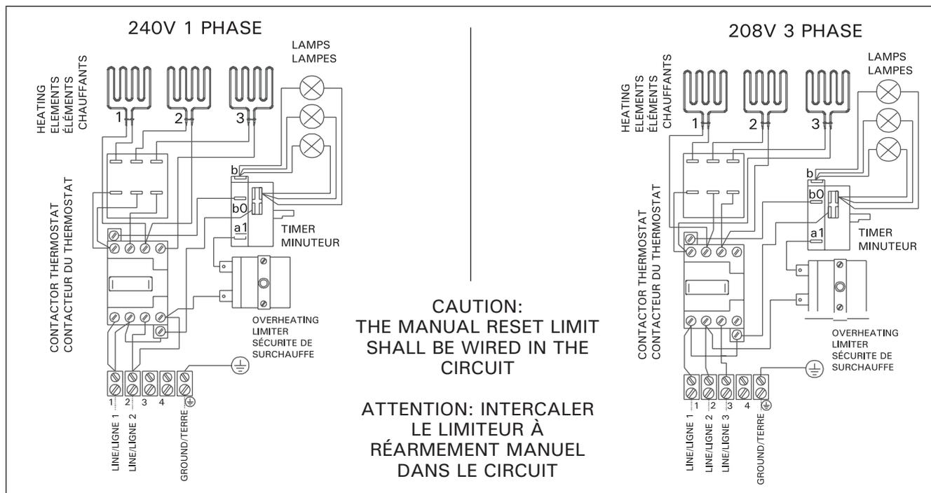
Figure 10. Electrical connections of the heaters KV-45, KV-60 and KV-80
