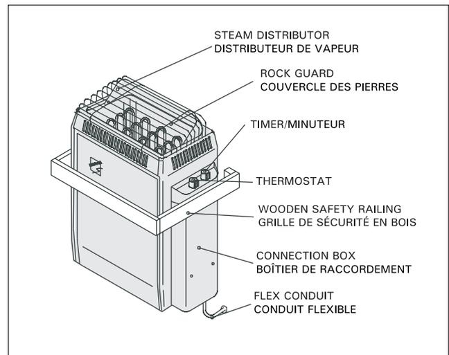
Figure 9. Connections and parts of the heater
