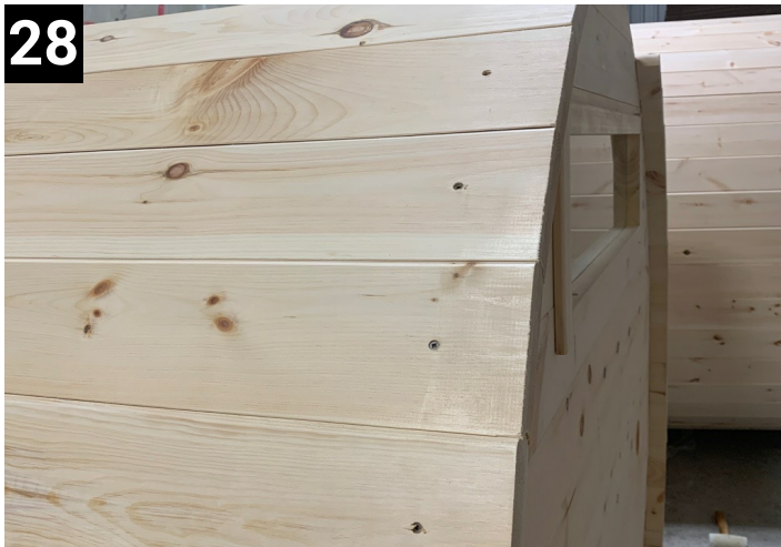
Put staves on and fasten on. Leave the last 8 staves unscrewed to allow putting in the top stave
