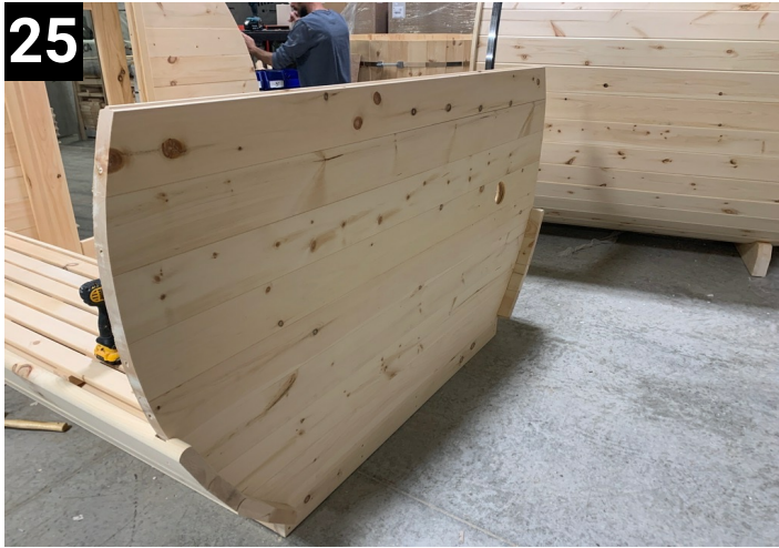
Add next back wall portion and fasten with 4" screws
