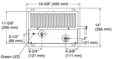
Minimum required access panel is 24" (610 mm) L x 15" (381 mm) H.
