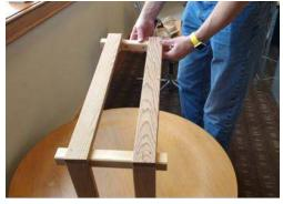
24. Attach the final piece—the remaining vertical fence post. When complete, position the fence around the heater and use the pre-drilled holes to attach it to the wall.
