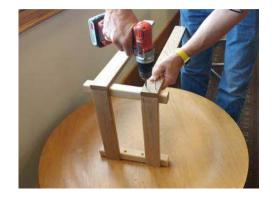
23. Prop up the pre-assembled portion and attach the two long horizontal pieces. Make sure the countersunk holes on the wall mounting bracket face inward.
