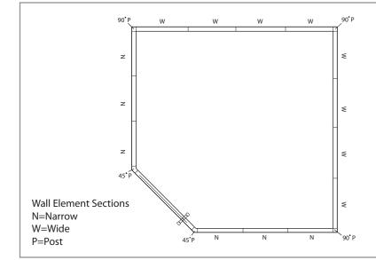
**STEP 2** - Locate the wall elements (sections). There are two sizes. The narrow element sections (N) are approximately 17" wide and will be used to construct the short walls that connect to the door. The wide element sections (W) are approximately 19" wide and will construct the two long walls.
