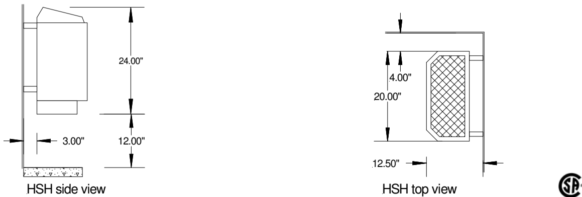
Figure 2. HSH clearances to wood surfaces
