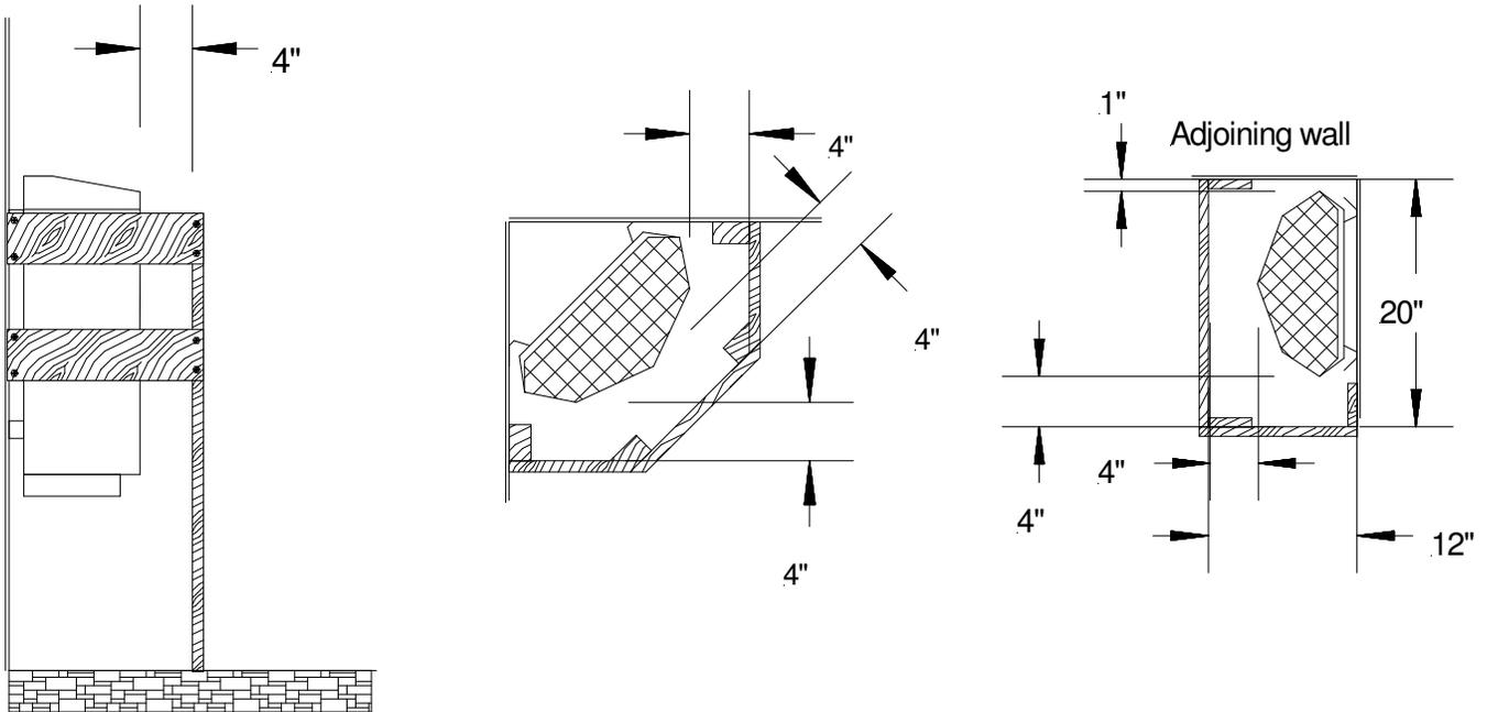
Figure 6. HSH heater guard clearances
