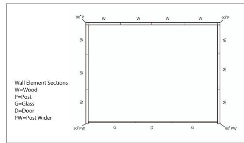
**STEP 2** - Locate the wood wall elements (sections). These will be inserted over the bottom rails as shown in the diagram.
