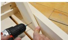
**STEP 28** - Assemble the lower bench by attaching the right and left framed leg supports to the bench and screwing into place with 4x60 screws. Be sure the two holes in the uprights are to the rear of the bench and the plastic floor protectors are down. Next, attach the angled support members so that the pins line up with the holes. Place a dab of wood glue (not included) in the holes before tapping into place. Secure the support members to the bench using 3.5x40 screws.
