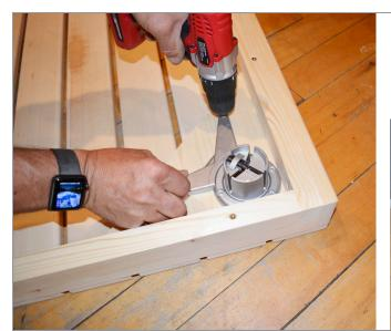
**STEP 22** - Attached the metal post support bracket to the bottom of the upper side bench using screws included in hardware packet. Slip the metal support post over the bracket and secure in place with the hex screw located in the support bracket.
